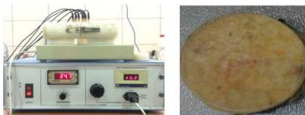
Fig.2: Heat transmission device and a tested sample
